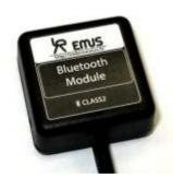
Emus Bluetooth module operates from 12V supply and communicates with Emus Control Unit via RS232 port (DISP.TX and DISP.RX pins). Connection is as follows:
